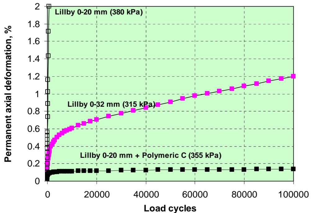
Figure 14. The permanent deformations developed in the Lillby aggregate test specimen during the permanent deformation test series performed after the freeze-thaw cycle. The constant confining pressure during the loading series was 50 kPa while the deviator stress was 300 kPa. The stress values presented in the parenthesis indicate the realised values of deviator stress during each test.
