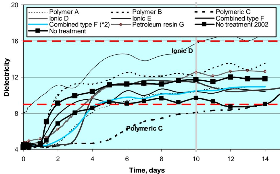
Figure 8. The TS test results obtained with the Troms aggregate. The test specimen 'No treatment 2002' was prepared earlier following a slightly different test procedure than what was used in connection with the other specimens.
