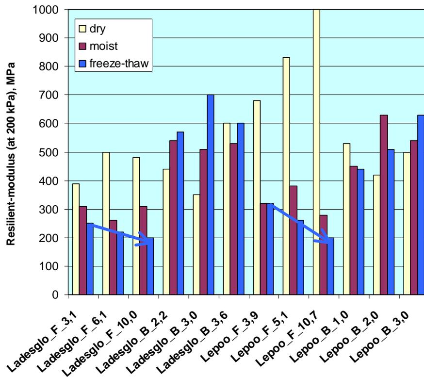
Figure 11. Resilient modulus values of the Lädenгло and Lepoo aggregates tested in dry condition, in moist condition and after a freeze-thaw cycle. The resilient modulus values correspond to the sum of principal stresses 200 kPa. Notation F means the fines content in a non-treated test specimen while B indicates the bitumen content in a treated test specimen. In the bitumen treated test specimen the fines contents were about 5 % for the Lädenгло aggregate and about 6 % for the Lepoo aggregate.
