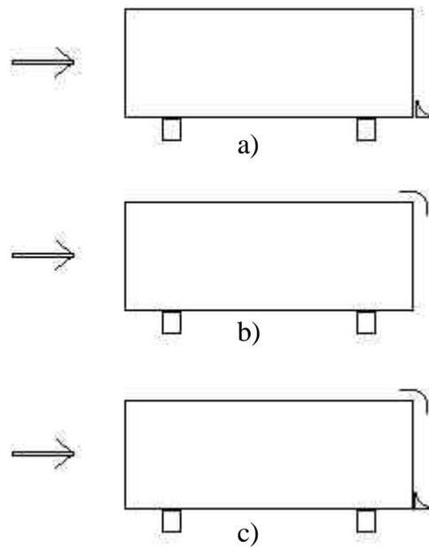
**Figure 4. Schematics of spoiler configurations used in sideview visualisations. a) bottom spoiler; b) top spoiler; c) top and bottom spoilers. Wind direction from left to right.**
