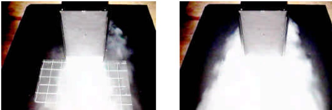
Figure 12. Snow smoke visualisation on model with sideskirts and sidespoilers. Left picture: sideskirts and side spoilers; Right picture: side spoilers only.
