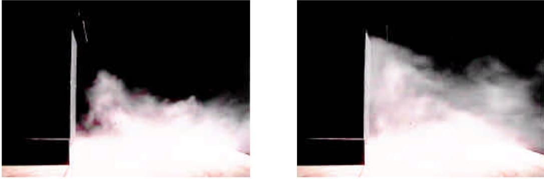
**Figure 8. Snow smoke visualisation of model with spoilers. Left: 90° bend spoiler; Right: 40° bend spoiler.**
