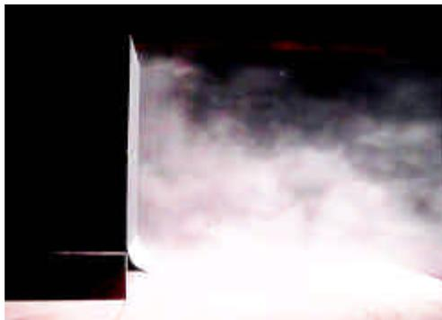
**Figure 9. Snow smoke visualisation on model with bottom spoiler.**
