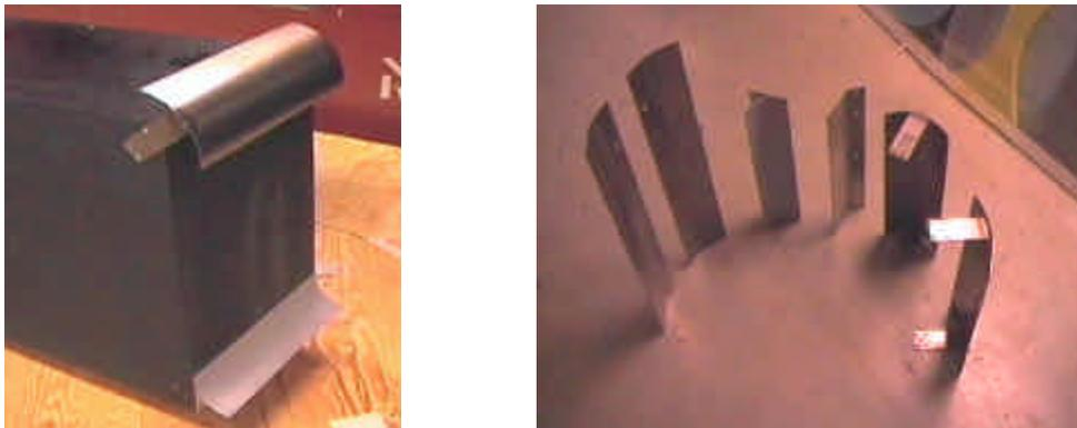
**Figure 5. Left picture: model with top and bottom spoilers; Right picture: photograph of the different spoilers. From left to right: sidespoilers, bottom spoiler, bottom front spiler, top spoilers.**
