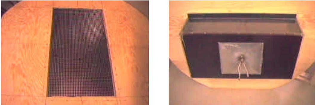
**Figure 3. Smoke chamber. Left picture: seen from inside the windtunnel; Right picture: seen from below.**
