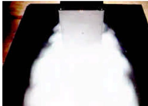
Visualisation of snow smoke behind a model of a heavy vehicle without spoilers.
