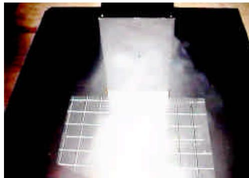
Visualisation of snow smoke behind a model of a heavy vehicle with spoilers.
