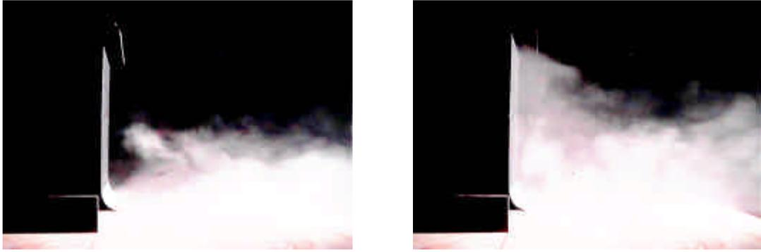
**Figure 10. Snow smoke visualisation on model with top and bottom spoilers. Left: 90° bend topspoiler; Right: 40° bend topspoiler.**
