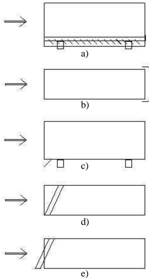
**Figure 6. Schematics of spoiler configurations used in topview visualisations. a) sideskirts (sideview); b) side spoilers (topview); c) bottom front spoiler (sideview); d) and e) bottom front spoiler in two different positions (topview).**
