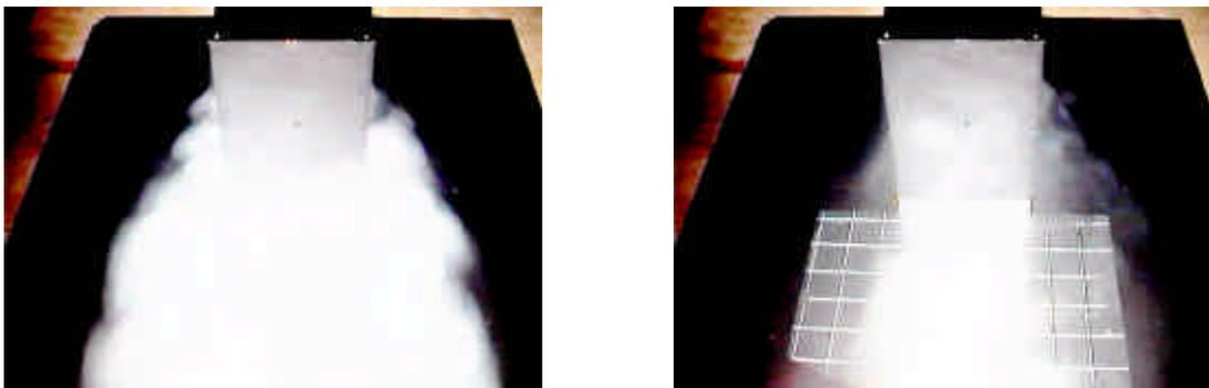
**Figure 11. Snow smoke visualisation on model with and without sideskirts (Right and left pictures, respectively).**
