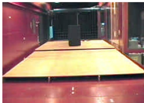
**Figure 2. View of the model and the false floor inside the wind tunnel**
