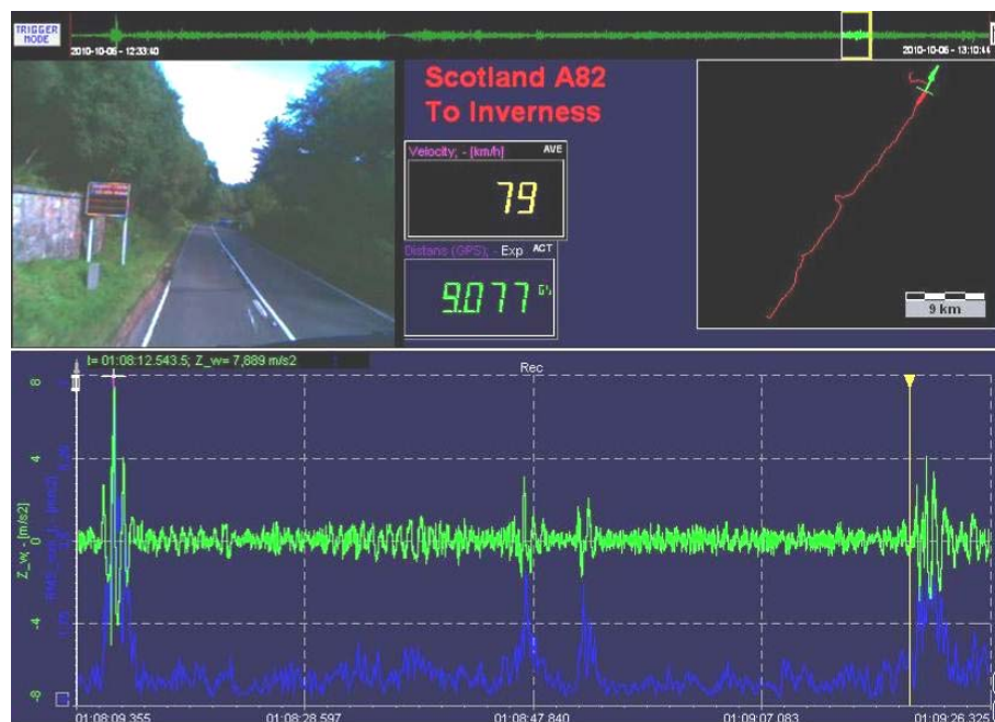
Figure 38 Impulse-response in the truck at a rough transversal joint on A82
