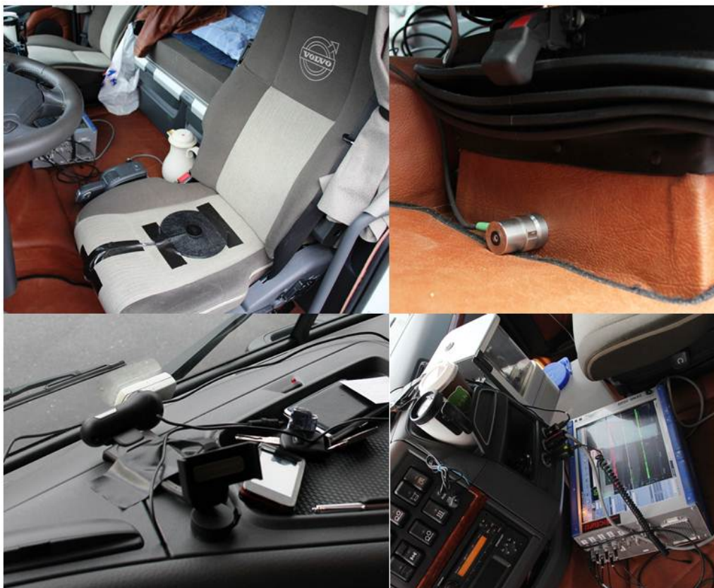
Figure 49 Instruments in the Volvo test truck used on European Highway E6 in Norway
