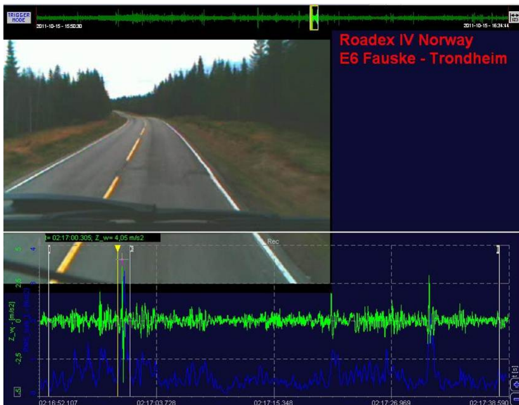
Figure 55 Mechanical shocks in the truck driver's seat at the old bad asphalt-joint
