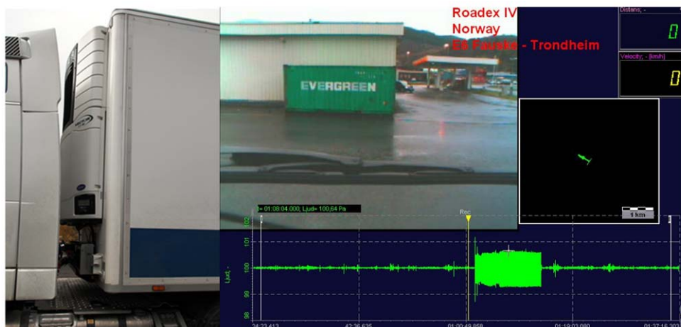
Figure 59 The driver's sleep can be disturbed by noise from the freight thermo-cooler
