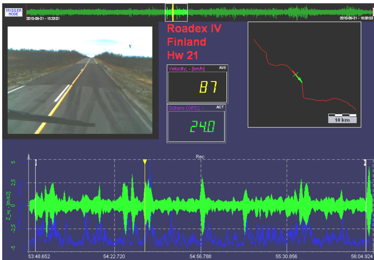
Figure 11 Patch repair zone at Highway 21: Intense mechanical shocks on the driver seat
