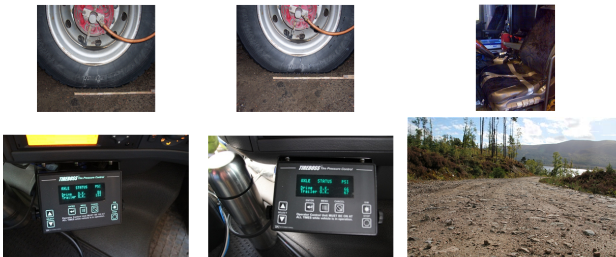
Figure 108 TPCS isolates the driver from mega-textured roads [Photo: J Granlund & P Granlund]
