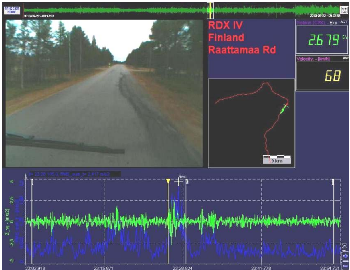
Figure 14 Intense truck ride vibration at deformed pavement edge on Road 956/957
