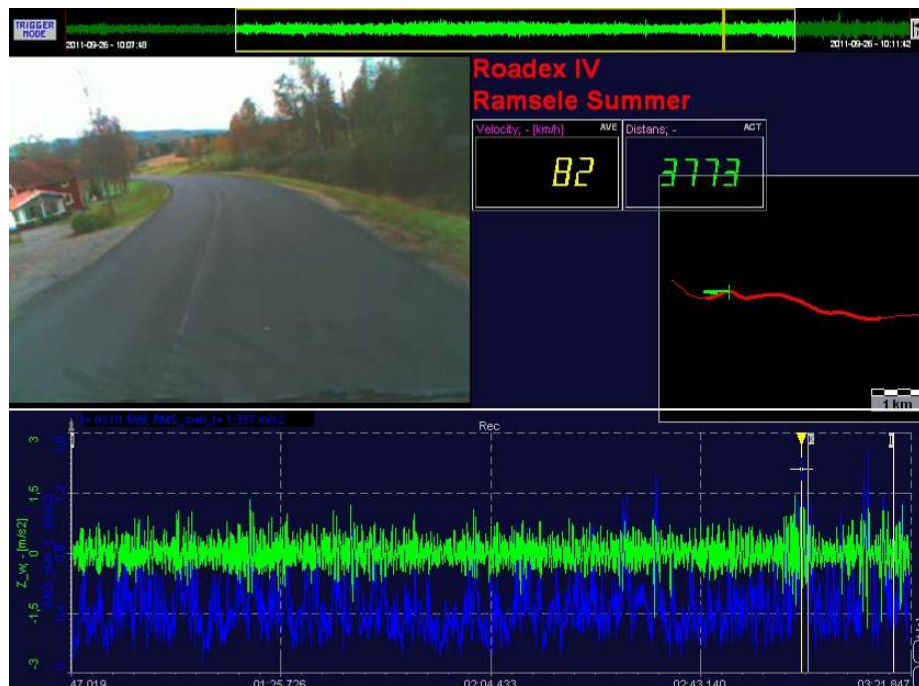
Figure 86 Road 1035 still gives a rough truck ride just after resurfacing 2011
