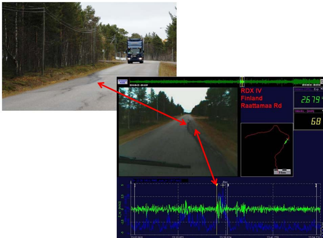
Figure 99 Pavement edge deformation is a common cause of road warpiness
