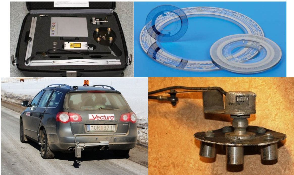
Figure 84 The portable LaserProf System and the odometer after being “killed” at a bump
