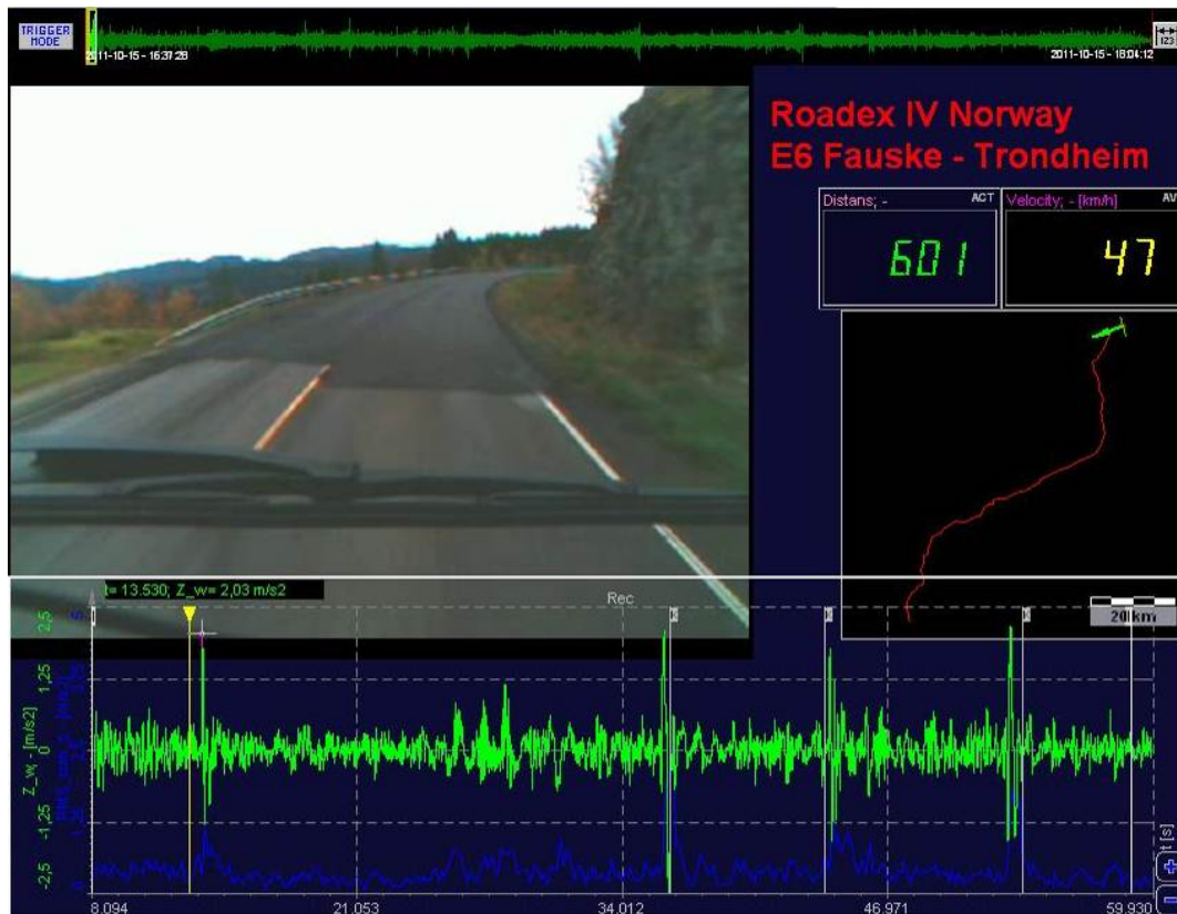
Figure 56 Mechanical shocks in the truck driver's seat at another bad asphalt-joint
