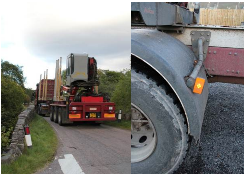
Figure 44 Narrow sections cause frequent scratching on tyre sidewalls and fenders
