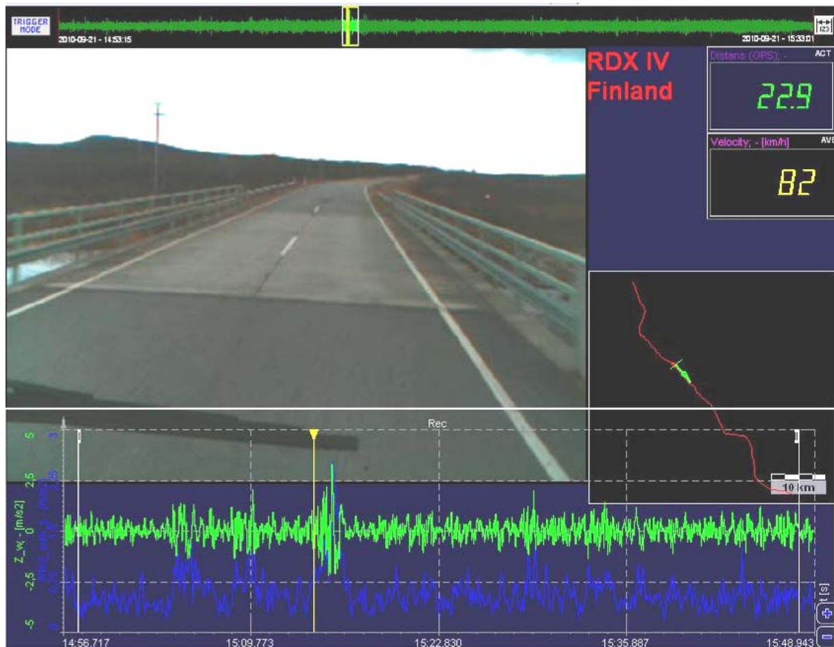
Figure 12 Intense ride vibration at an improper bridge backfill
