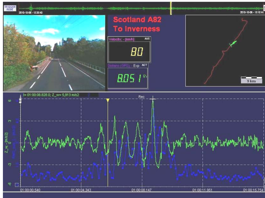
Figure 36 The truck incurred severe bumps on a bridge on the A82 bound for Inverness
