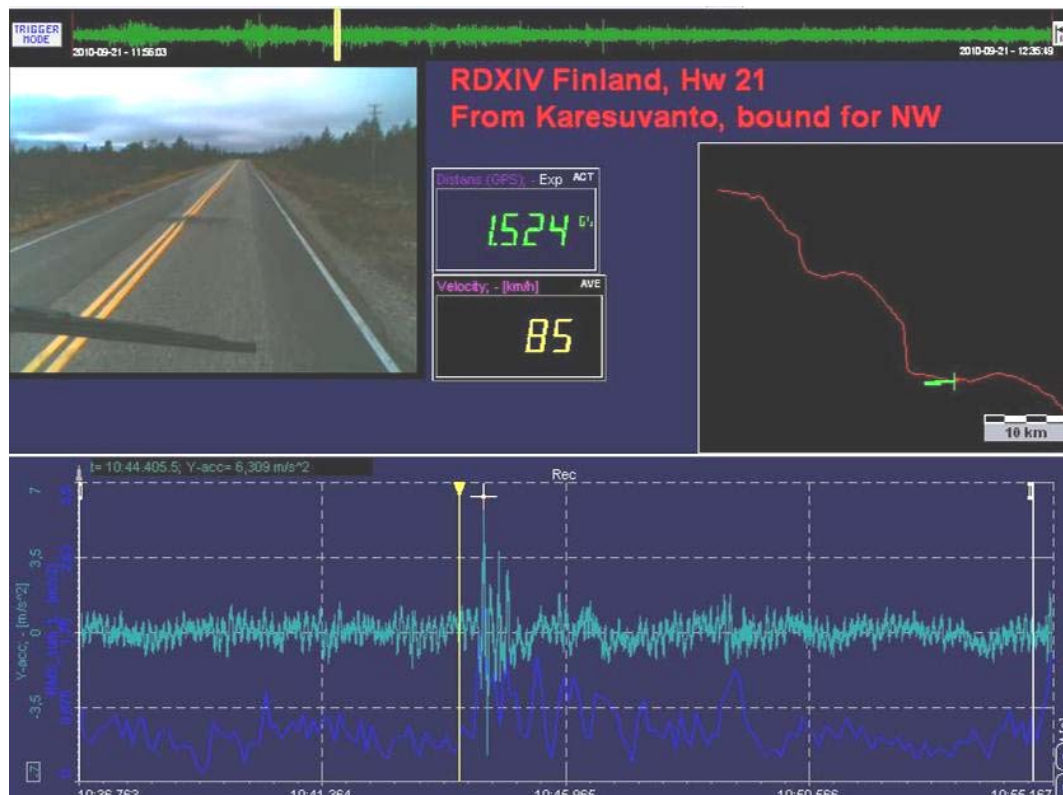
Figure 17 Lateral buffeting of test truck at a rising boulder on the road centreline on Highway 21
