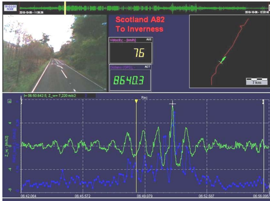
Figure 39 The truck suspension shows resonance at low frequencies / long wave unevenness
