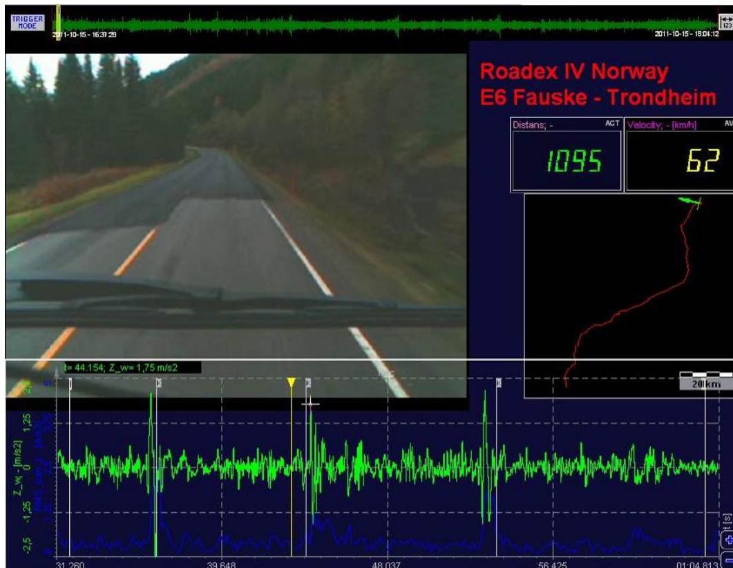
Figure 54 Mechanical shocks in the truck driver's seat at a bad asphalt-joint
