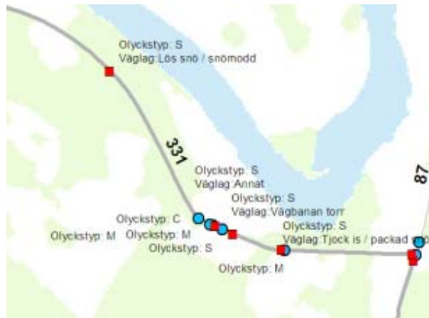
Figure 90 Crashes have clustered at the improperly banked Roos curve
