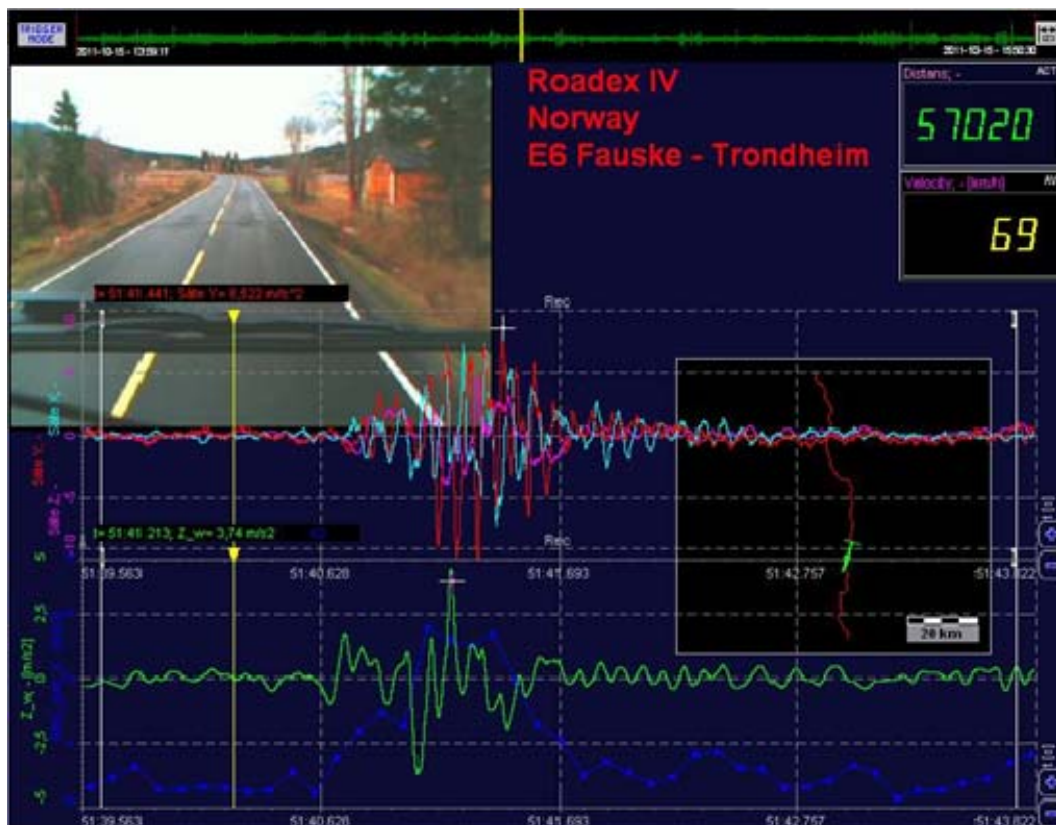
Figure 57 Bumpy truck ride due to settlements at a culvert
