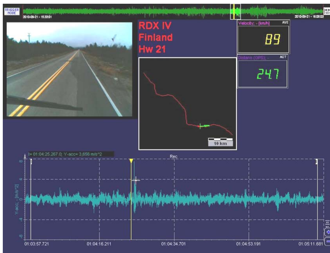
Figure 16 Hazardous lateral truck vibration at deformed pavement edge on Highway 21
