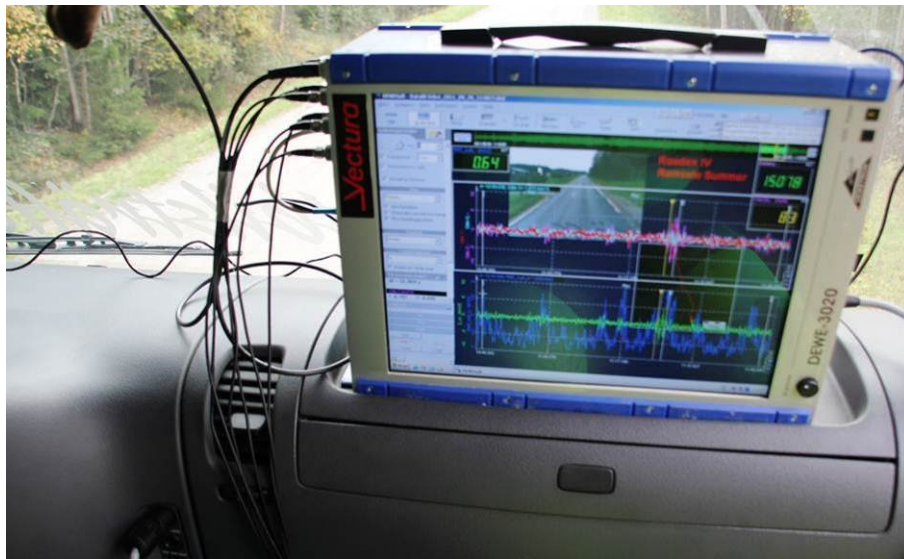
Figure 2 A Dewetron 3020 is the heart of Vectura’s ride quality measurement system
