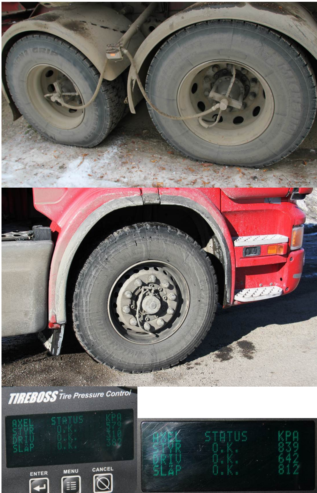
Figure 75 The TPCS controls all tyres on Brorssons truck, including on the steer axle
