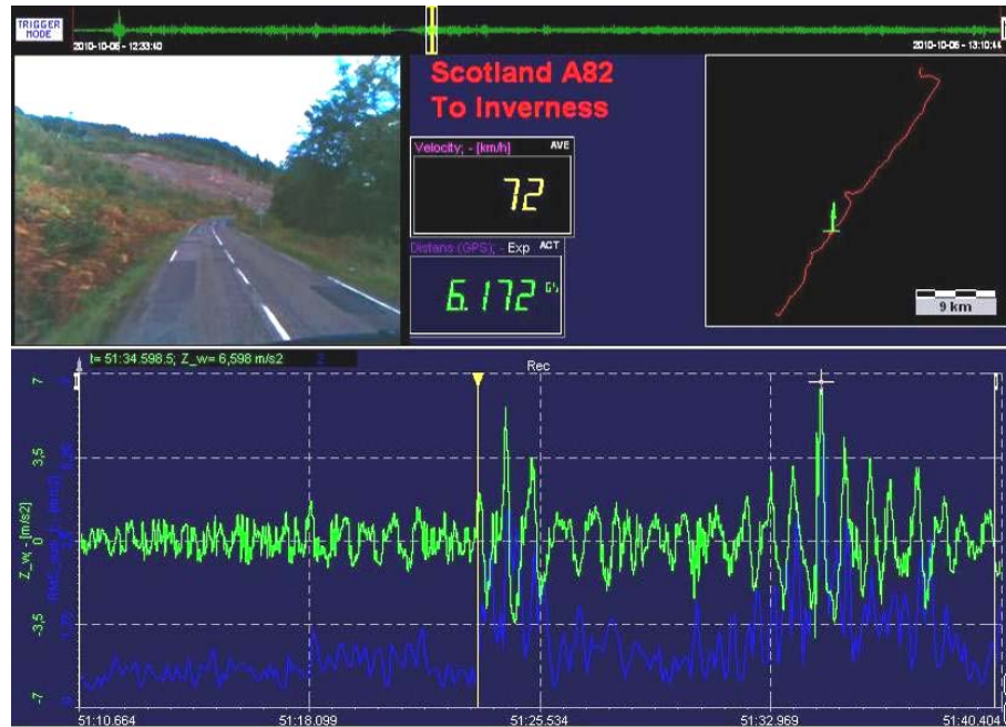
Figure 37 Rough truck ride over patches on A82 bound for Inverness
