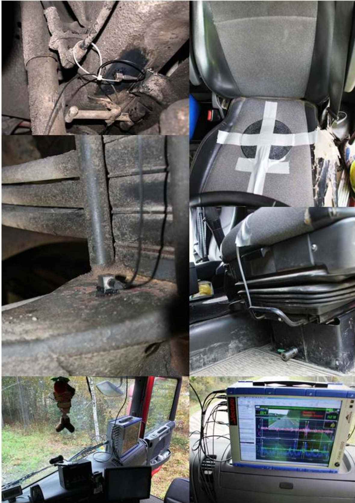
Figure 76 Instrumentation in the Scania test truck
