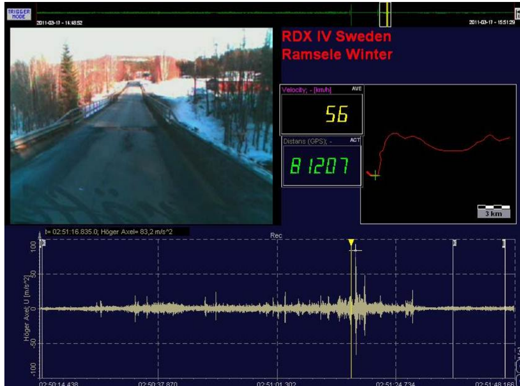
Figure 81 High acceleration of the truck wheel assembly at settlement in bridge backfill
