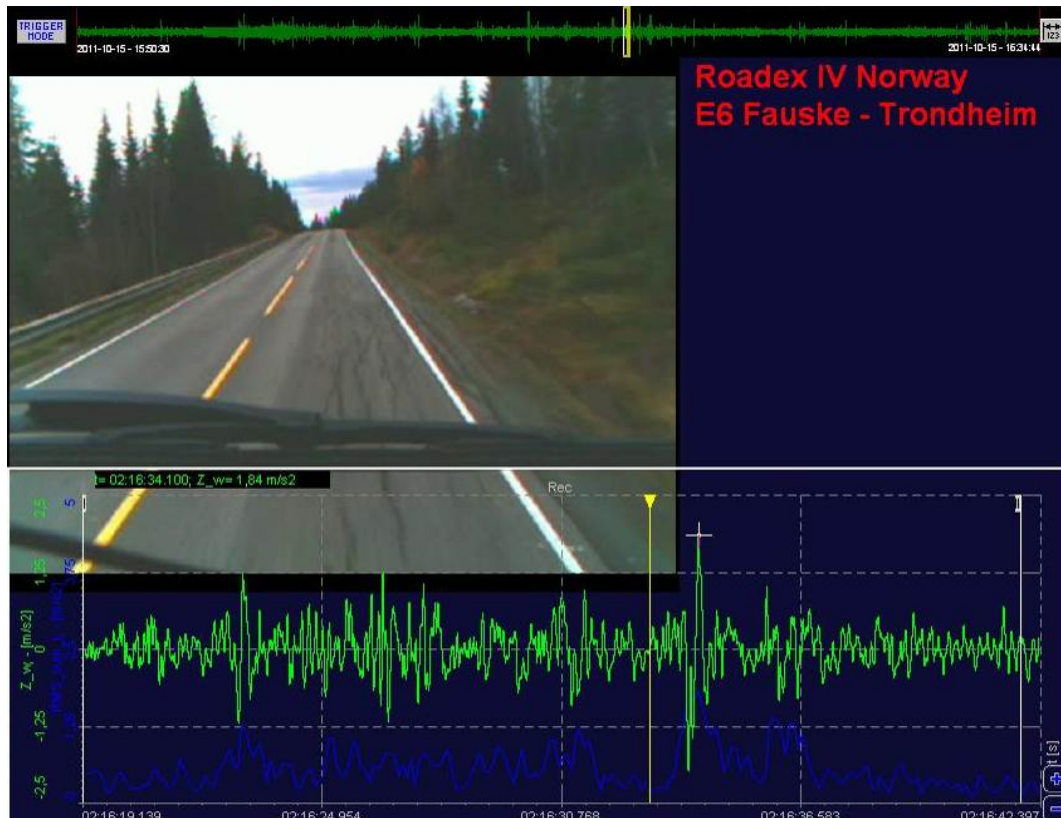
Figure 58 Bumpy truck ride at a deformed and alligator-cracked weak pavement section
