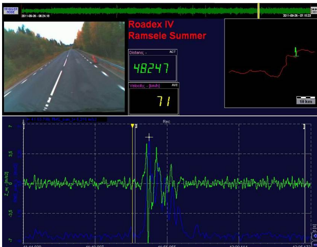
Figure 87 Transient vibration at an edge deformation on a newly repaired section of Road 335
