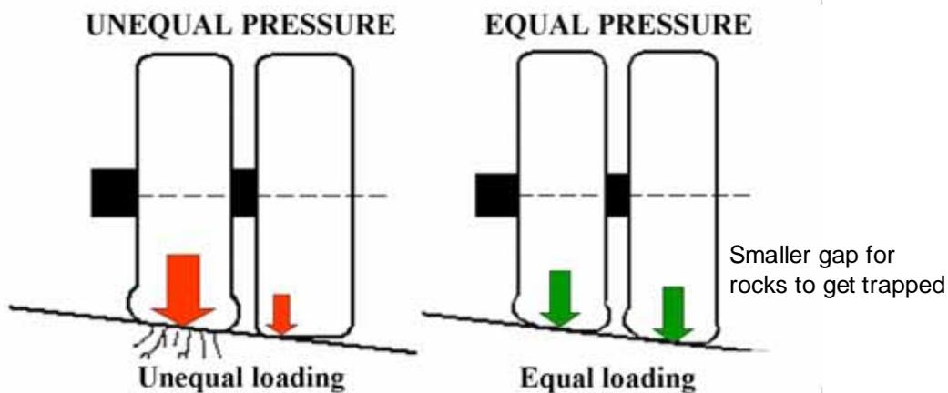
**Figure 2.3 Effect of equal pressure in twin tyres on a crowned road (TPC International)**
