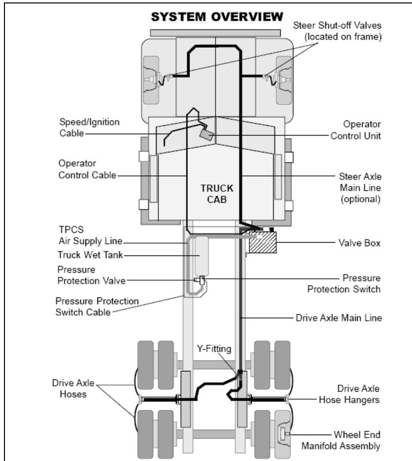
**Figure 3.6 Schematic diagram of a TPC system on a tractor unit (TPC International)**
