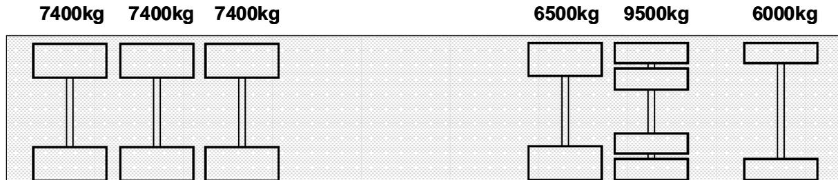
**Figure 4.3** Schematic of James Jones TPCS 6x2 TAG unit with super single tri-axle trailer
