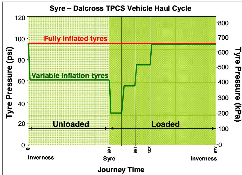
**Figure 3.4** Test vehicle haul cycle from forest to Norbord processing plant, Dalcross, Inverness
