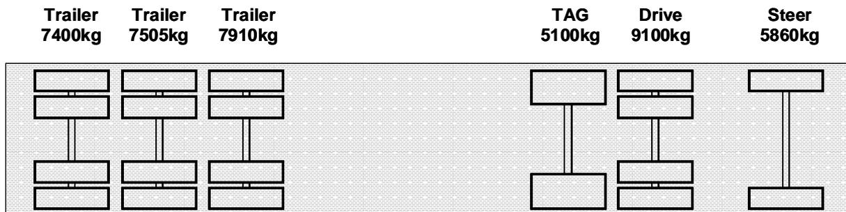
**Figure 3.2** Schematic of underside of the loaded test vehicle showing the measured axle loads in kg
