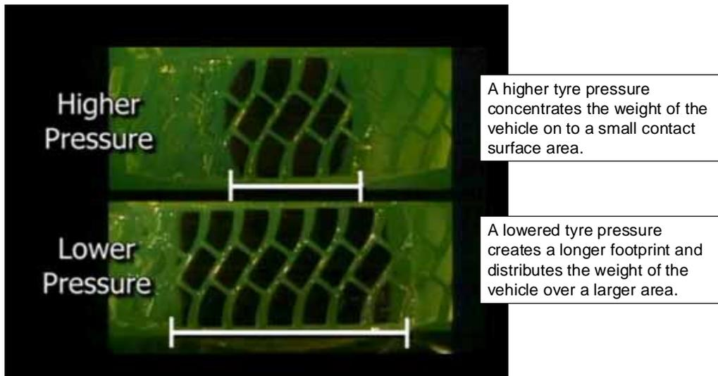
**Figure 2.2 Lengthening the footprint of a radial tyre by lowering its inflation pressure (TPC International)**
