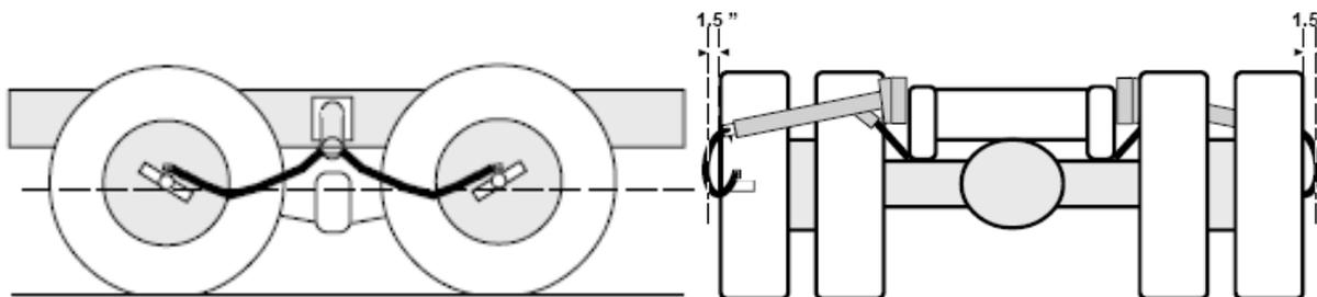
**Figure 3.7 Schematic diagrams of a TPCS air hose arrangements on a tractor unit (TPC International)**
