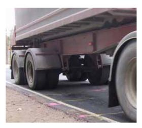
Figure 11. Twin tyres are still mainly used in Northern Periphery area.
