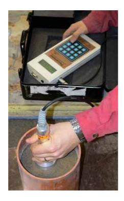
*Figure 7. Measurement of the dielectric value and electrical conductivity of the upper part of the Tube Suction test specimen.*
