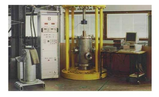
Figure 10. Large scale repeated load triaxial test facility developed at the Tampere University of Technology.
