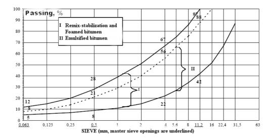
Figure 5. The range of grain size distribution of the materials suitable for bitumen stabilisation according to the Finnish design codes (Tiehallinto 2002).
