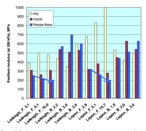
Figure 11. Resilient modulus values of the Lädesglo and Lepoo aggregates tested in dry condition, in moist condition and after a freeze-thaw cycle. The resilient modulus values correspond to the sum of principal stresses 200 kPa. Notation F means the fines content in a non-treated test specimen while B indicates the bitumen content in a treated test specimen. In the bitumen treated test specimen the fines contents were about 5 % for the Lädesglo aggregate and about 6 % for the Lepoo aggregate.
