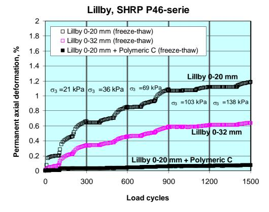
Figure 13. The permanent deformations measured during the resilient deformation test performed after the freeze-thaw cycle in the test specimens made of Lillby aggregate.
