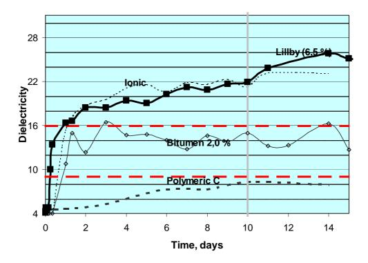
*Figure 9. The dielectric values determined in the TS tests performed with Lillby crushed rock aggregate.*
