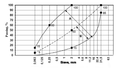
Figure 4. The range of grain size distribution of the materials suitable for cement stabilisation (area B) according to the Finnish design codes (Tiehallinto 2002).
