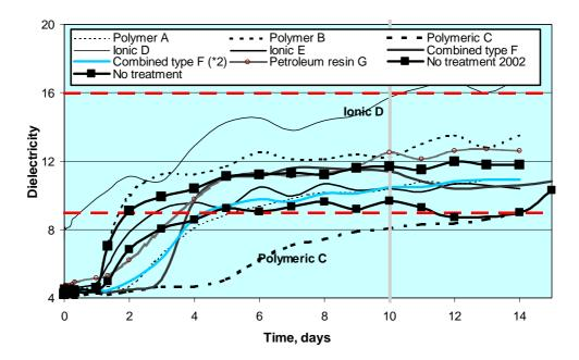
Figure 8. The TS test results obtained with the Troms aggregate. The test specimen 'No treatment 2002' was prepared earlier following a slightly different test procedure than what was used in connection with the other specimens.
