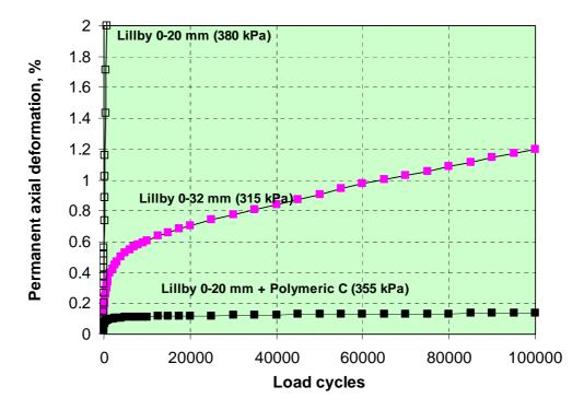
Figure 14. The permanent deformations developed in the Lillby aggregate test specimen during the permanent deformation test series performed after the freeze-thaw cycle. The constant confining pressure during the loading series was 50 kPa while the deviator stress was 300 kPa. The stress values presented in the parenthesis indicate the realised values of deviator stress during each test.
