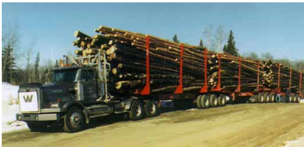
Figure 129. Forestry sector partnership experimental Twelve-Axle B-Train used in Saskatchewan Rural Partnership Haul Program (photo Curtis Berthelot)
