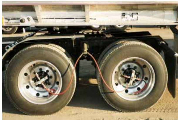
Figure 127. CTI system installed on a dual tandem wheel (photo courtesy of Curtis Berthelot)
