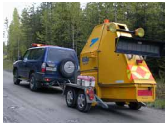
Figure 40. Finnish Road Enterprise Falling Weight Deflectometer unit used in Roadex II surveys.
