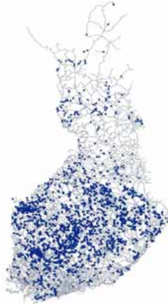
Figure 4. Public gravel roads with spring thaw problems in Finland (Virtala 2004).
