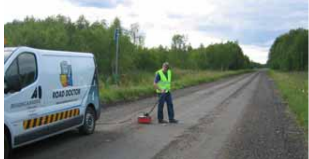
Figure 39. Measuring GPR cross sections at the Ängesby test site in Sweden using a 400 MHz ground coupled antenna.
