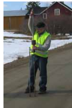
Figure 42. DCP tests at Kemijärvi test site in spring 2004 using the Norwegian DCP system.
