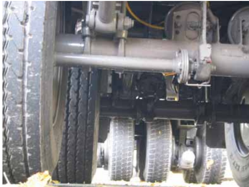
Figure 131. Axle configuration of a Low Ground Pressure Vehicle spreads much of the vehicle load onto the road centre.
