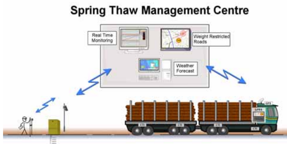
Figure 27. Schematic description of technique for managing spring thaw weakening (Saarenketo and Aho 2005) (see also chapter 11.2)
