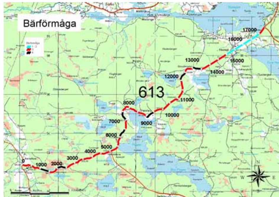
Figure 4. Example of a GIS map presenting bearing capacity results on road 613 in Gävleborg county.
