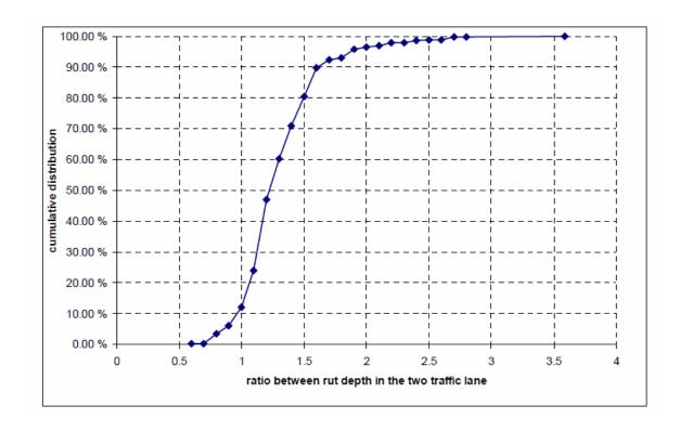
The diagram shows the rutting ratio between the two traffic lanes in sloping ground
