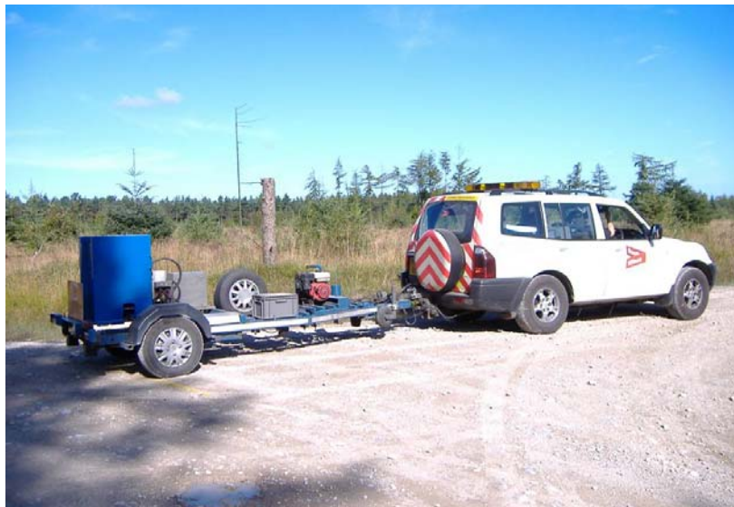
Figure 3-2 The Falling Weight Deflectometer Equipment
