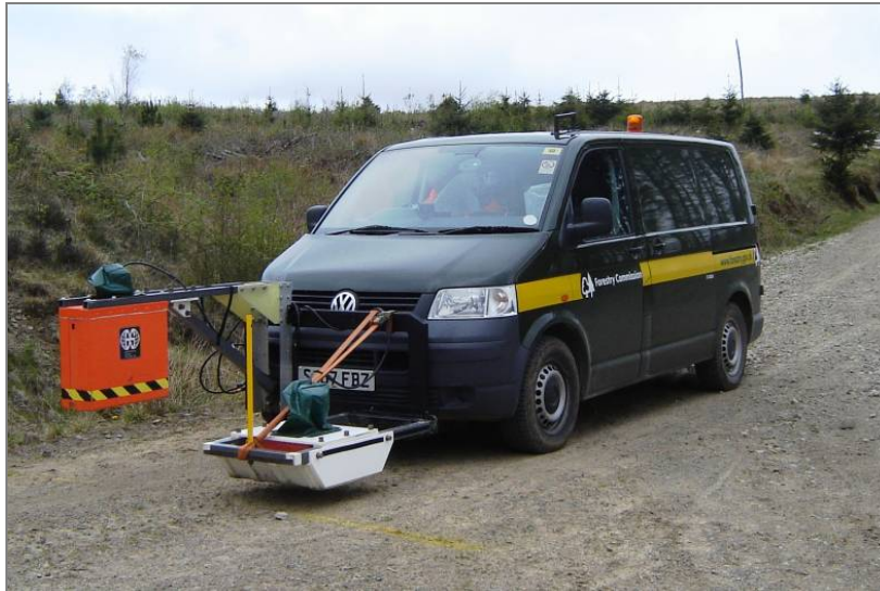
Figure 3-1 The Forestry Commission Road Condition Survey vehicle
