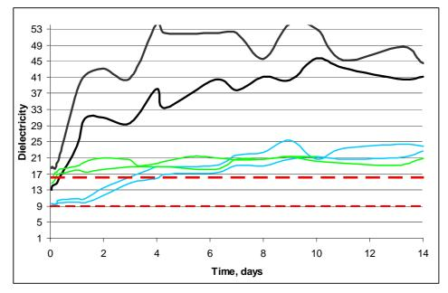
Image 4.4. Tube Suction test dielectricity graphs for untreated (black) and treated (coloured) aggregate from the local road 19735.
