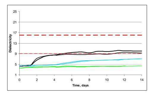
Figure 4.2. Tube Suction test dielectricity graphs for untreated (black) and treated (coloured) aggregate from the local road 13581.
