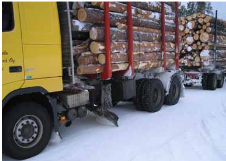
Figure 5. Under blade mounted on a timber truck in Finland that is also used for winter maintenance of forest roads.
