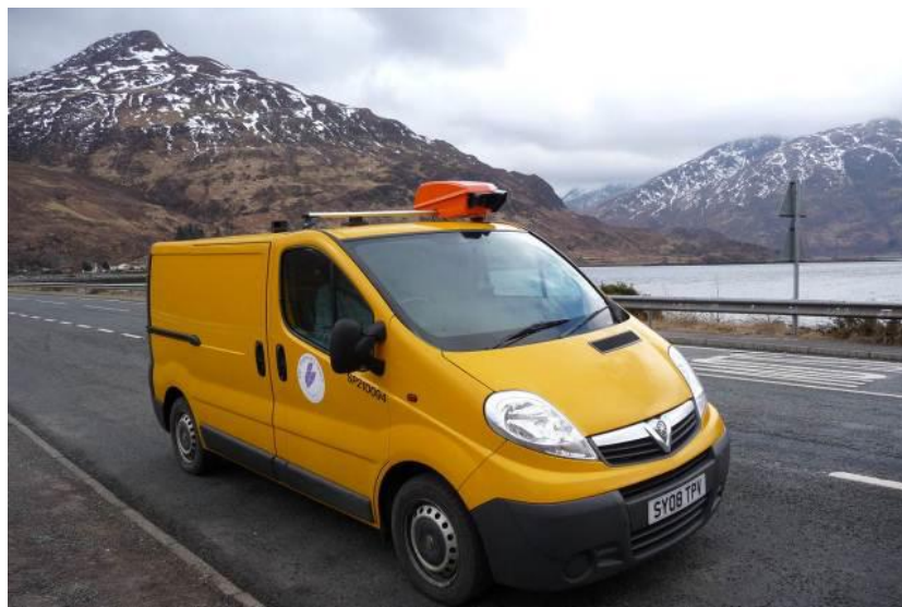
Figure 3.7.1. Digital cameras and GPS are normally placed on the roof of the survey vehicle for drainage analysis. Vehicle used in the Highland region of Scotland.
