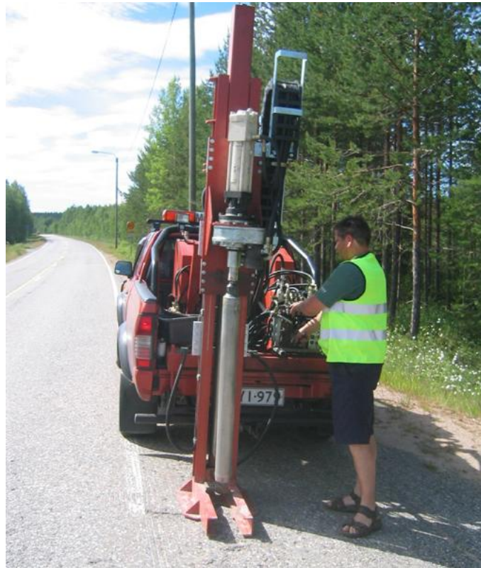
Figure 3.3.1. Drilling a sample of the top part of the pavement structure
