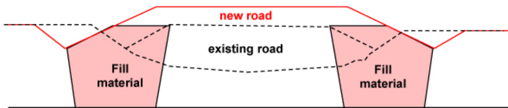
Figure 4.5.1. Diagram of road cross-section widened by excavating and replacing on each side of the existing road – the "legs" widening
