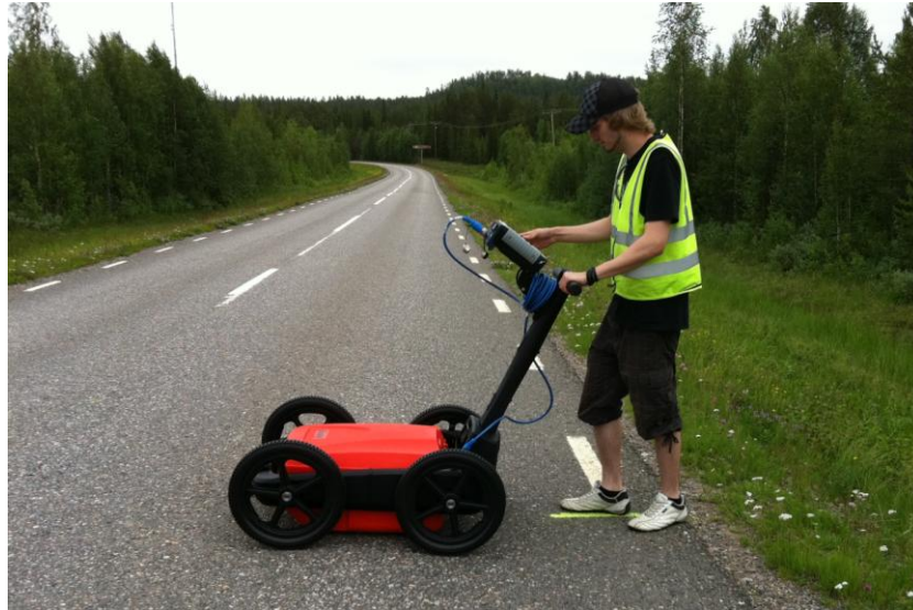
Figure 3.2.1. Cross section measurement with GPR provides excellent information about the road structures in the transverse direction.
