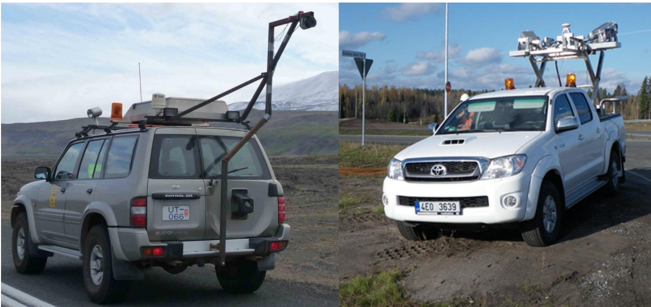
Figure 3.6.1. Everyman's RDLs Laser scanner survey vehicle (left) and a high precision Quantum 3D laser scanner survey vehicle (right) used in ROADDEX surveys
