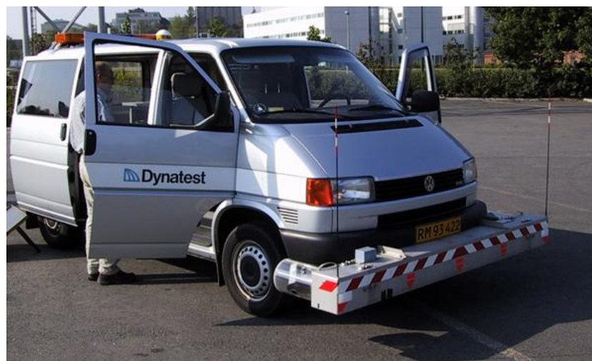
Figure 3.8.1. Survey van equipped with laser profilometer for roughness and rutting measurement
