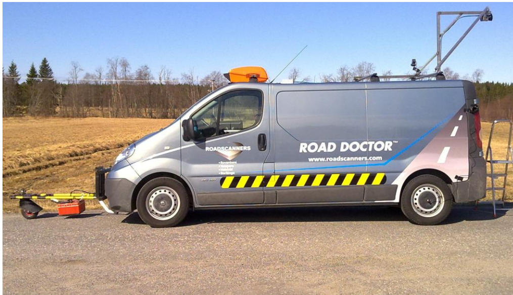
Figure 3.4. The survey van equipped with laser scanner at the back (high above the roof) and a 400 MHz ground coupled antenna at the front of the van. The orange box on the front of the roof is the CamLink video-logging system.
