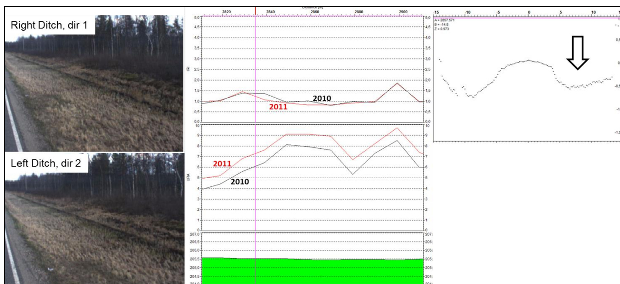
Figure 433_3. Example from road 80, section 11, chainage 2020 m. The cross section (top right) from the right ditch shows that the bottom level of the ditch is only about 50 cm from the road profile and clogged with vegetation, which is preventing water flow. The elevation frame (bottom middle) shows how flat the topography is in the area. The rutting values from 2011 (second graph in the middle) have grown evenly by about 1 mm from the results of 2010. The maximum rutting values are about 10 mm at this point. The IRI values (top middle) are about 2.0 mm at the highest.
