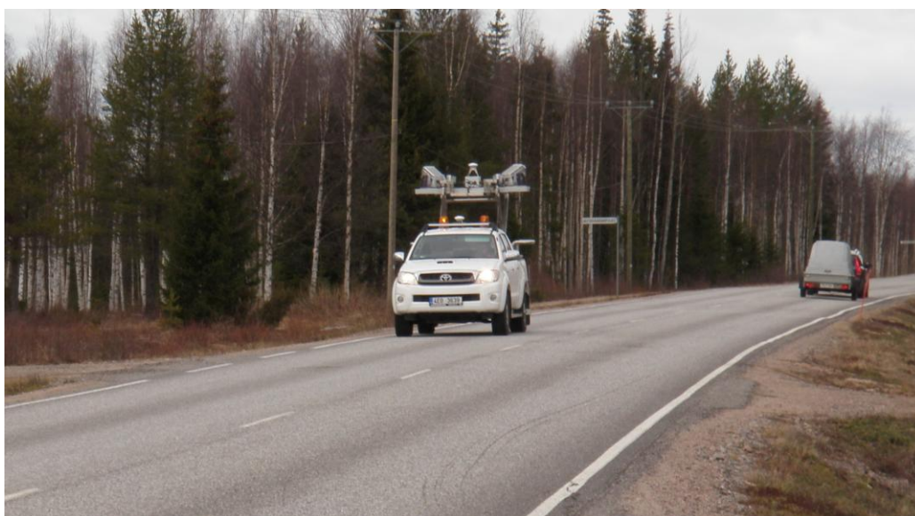
Figure 3.5. The Quantum 3D laser scanner survey vehicle of GEOVAP Ltd measuring road 934 in April 2011.
