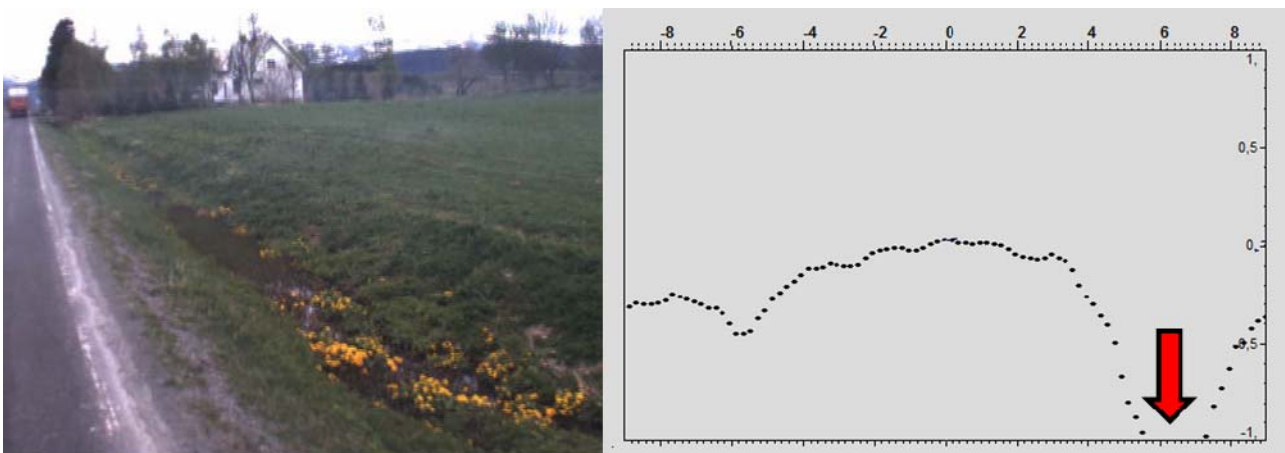
Figure 43: Vegetation was slowing down the water flow at chainage 25220m, good depth on the right ditch though. Laser scanner shows that the ditch on the left side is too shallow. Severe deformation problems can also be seen on the road.
