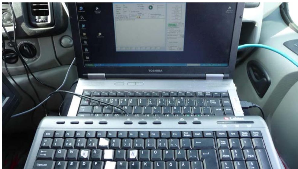
Figure 4: Keyboard (front) was used for drainage analysis, pieces of paper helped to choose the right keys during the survey. Laptop (back) was used to collect the laser scanner data.
