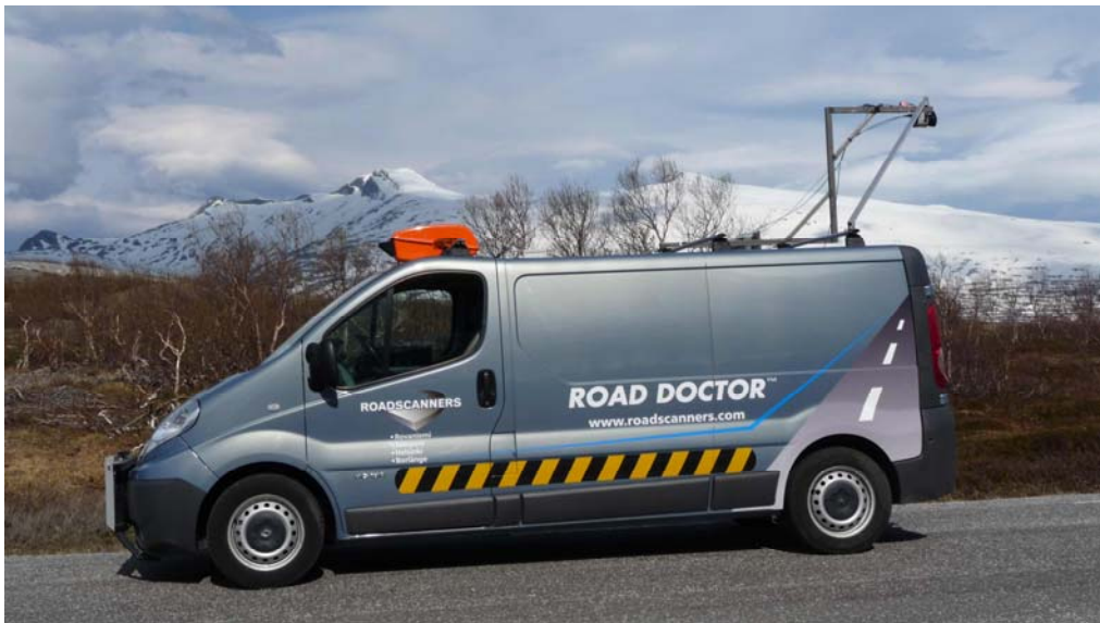
Figure 3: The survey vehicle used in the project. Video cameras were placed in the orange CamLink box for shelter from the rain and dust.
