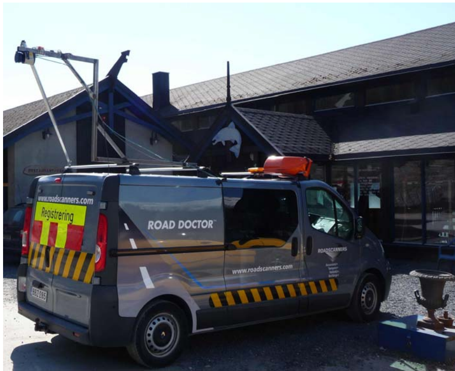
Figure 5: The laser scanner behind the survey vehicle at the height of 3m.
