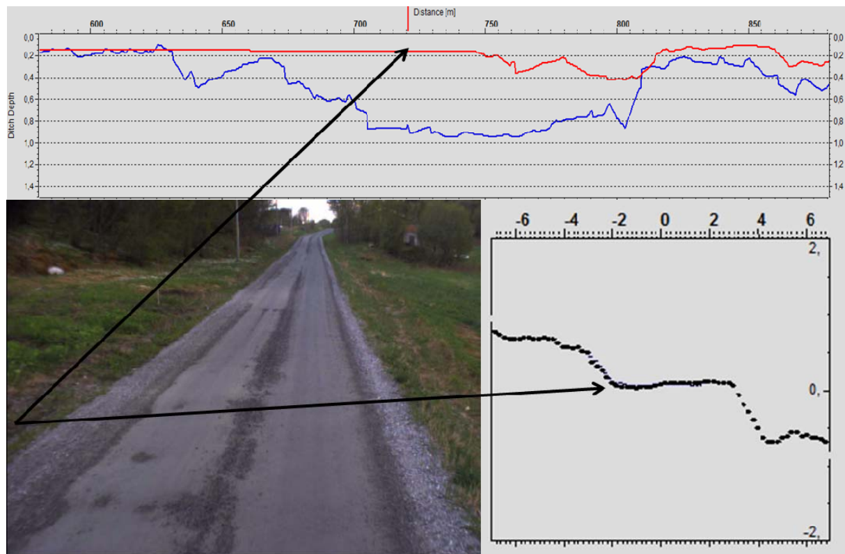
Figure 63: On the upper side of the slope the ditch was inadequate which is seen both on ditch depth data (top field) and on cross section data (lower arrow). Chainage 722m.
