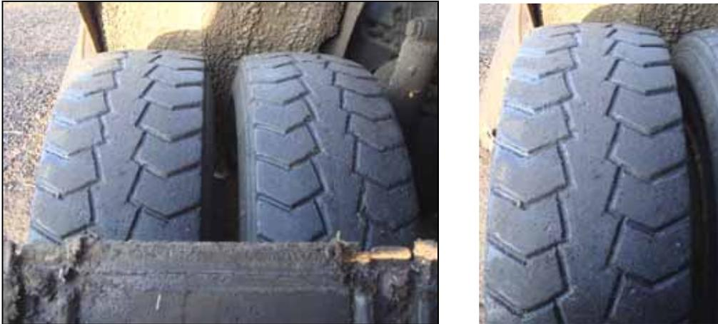
**Figure 4.5 Photographs of the condition of the drive tyres of the test vehicle on 9 February 2008**
