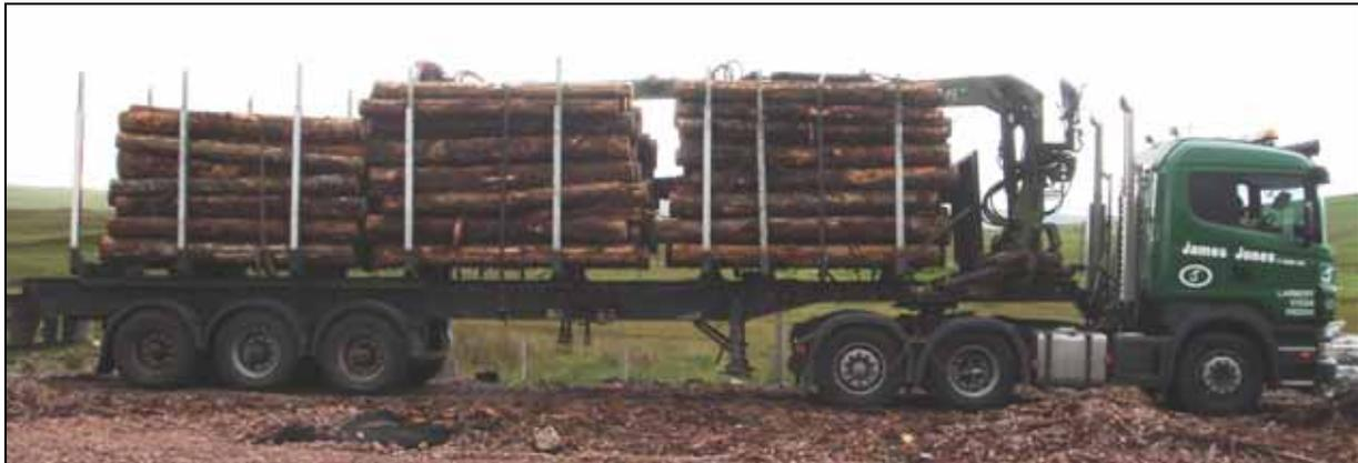
**Figure 4.2** Photograph of the loaded James Jones TPCS 6x2 TAG unit with super single tri-axle trailer during hauling operation on the A897 public Road, July 2007
