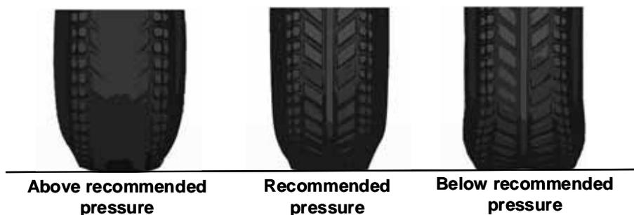
*Figure 2.1 Diagrams showing effects of over and under-inflated tyres (courtesy of Michelin UK)*
