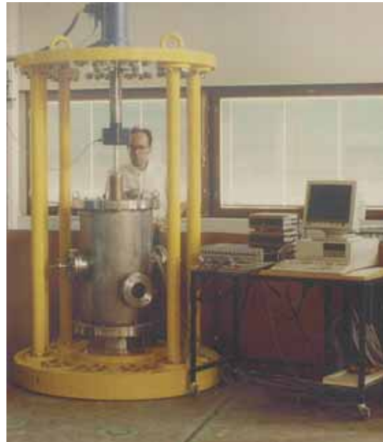
Figure 24. Repeated Load Triaxial Test Facility at Tampere University of Technology for 200 & 300 mm diameter specimens
