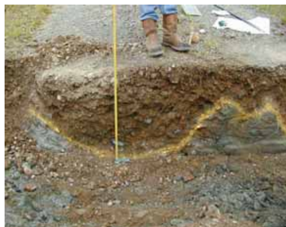
Figure 12. An advanced case of Mode 2 rutting seen in an exhumed pavement with a very weak subgrade. (photo: courtesy W Tyrrell)
