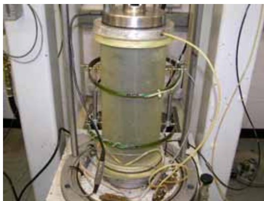
Figure 23. Specimen ready for testing in University of Nottingham triaxial apparatus.
