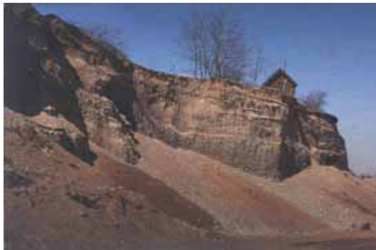
Figure 16. Glacial gravels being excavated from an esker deposit, Sweden.
