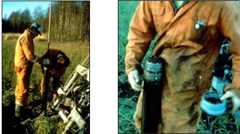
Figure 15. Photographs of The Swedish Geotechnical Institute Sampler in use. Source: Swedish Geotechnical Institute.
